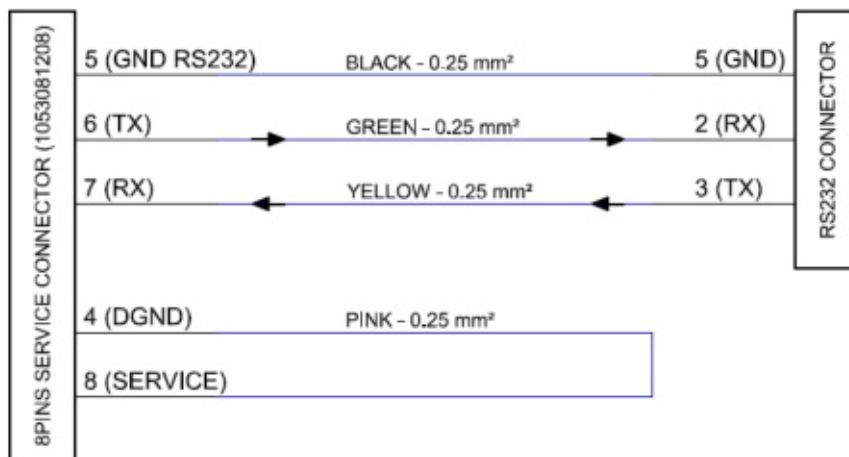
RS232 CONNECTOR (DB9) - FEMALE, WIRING VIEW
